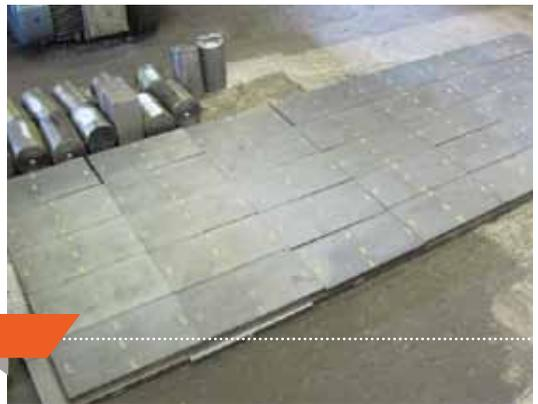
The electroslag remelting process allows reaching very high cleanliness which is the key factor in mouldmaking with economical advantages over other refining methods. Ingots are obtained with purity levels that were unknown a few years ago leaving behind prejudices as the process is evolving. Also, in efforts to cutting lead times, ESR process eliminates any conditioning of ingots prior to remelting steps and following forging steps.
