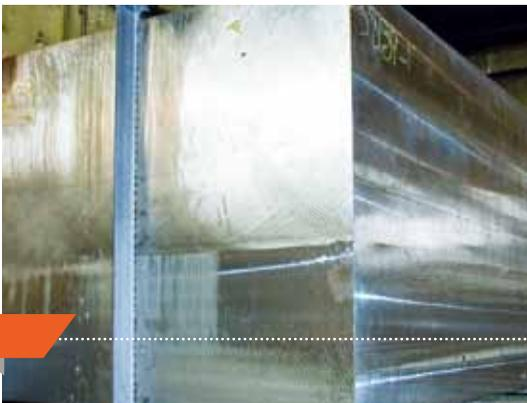
quality steel to insure a flawless surface on the final product. **SF-2000 LQ40 ESR** is the latest development in the **SF-2000** family at Sorel Forge. It is an electroslag remelted lens quality mould steel with cross section hardness of 40 HRC showcasing optimal cleanliness for mirror polishing capability giving the mouldmakers the possibility to manufacture the vision of designers.
